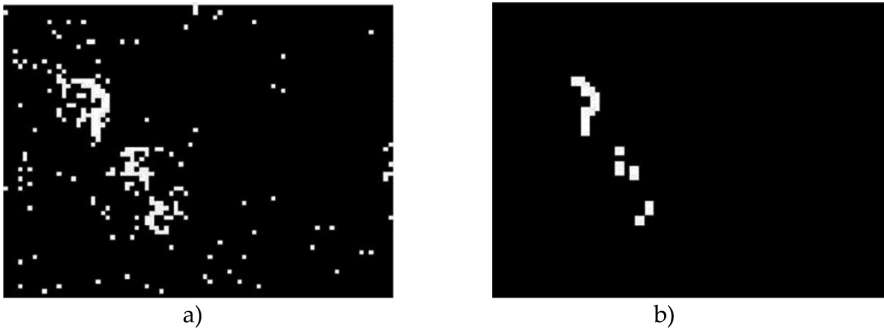
Fig. 7. The example of noise reduction based on the morphological operations: (a) the original binary image and (b) the image after applying the opening operation
